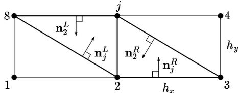
Figure 6: Stencil C for the coefficient of  $u_2$ .
