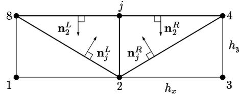
Figure 7: Stencil D for the coefficient of  $u_2$ .
